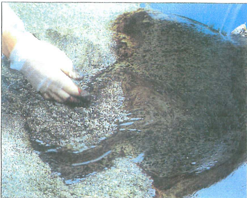
Figure 2 Oil globules of trapped crude oil and CytoSol biosolvent float out of sand as rinse water is applied
